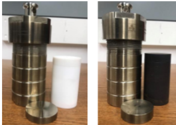
Fig.4. Hydrothermal autoclave (a) white teflon lined (left) (b) black teflon lined reactors at GL
