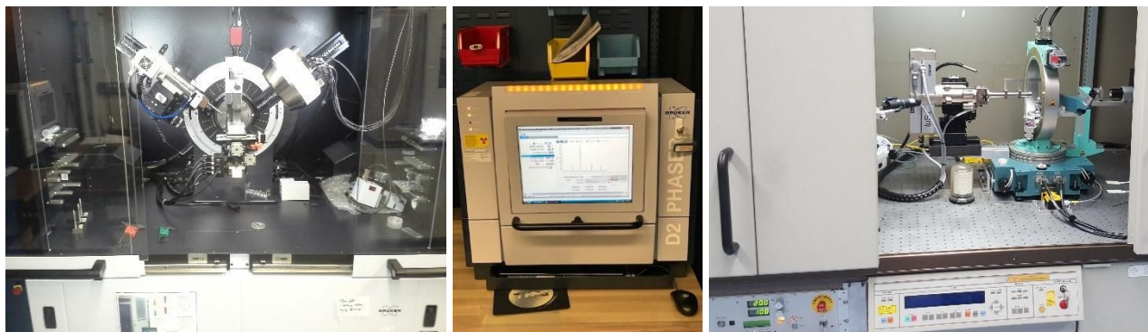
X-ray Diffractometers at GL. Left – Bruker D8; center – Bruker D2 phaser (powder), right – “Ingaku” (single crystal)
